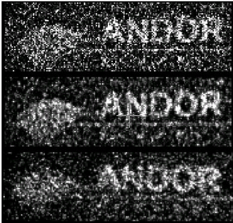
Figure 9. The top image is the EMCCD and the bottom image is the ICCD, the middle image is the EMCCD spatially smoothed using data of Figure 1. The average signal level of the white areas are approximately three electrons/pixel for all 3 images and gains for both systems were approximately X1800 each.
