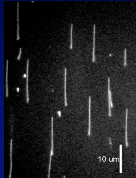
DNA strand metallized with palladium bridging two gold electrodes (group of M. Mertig and W. Pompe, TU Dresden)
